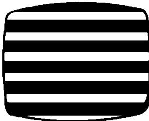
FIG. 3. HORIZONTAL BARS PRODUCED BY 400 CPS MODULATION ON SCREEN OF TV RECEIVER
